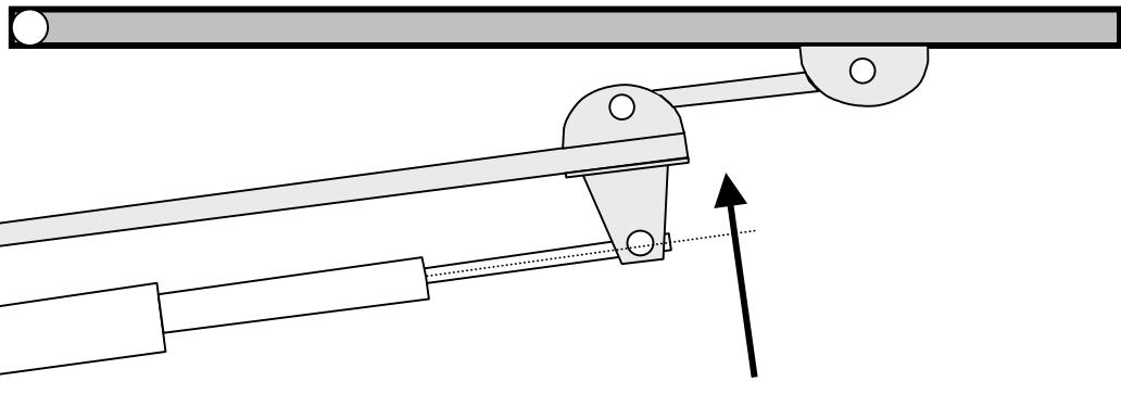
**PLAQUER L'ENSEMBLE PANTOGRAPHHE , BIELLETTE, DEMI LUNE, SUR LE PORTAIL ET FIXER
